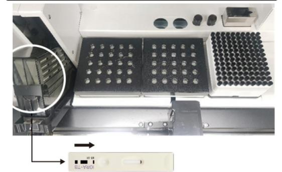
1. Load the cartridges, Detector tubes, Diluent, tips and ID chip in the instrument.
