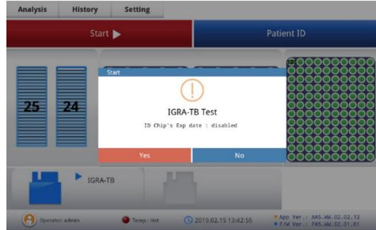
7. Confirm the agreement between test item and a program on the instrument. If correct, Press "Yes" on the screen.
