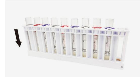
3. Load the processed tubes into the tube rack sequentially.
