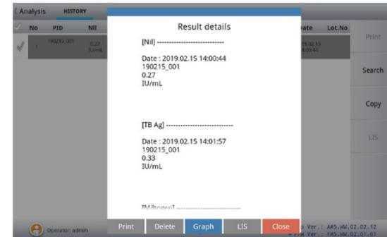
9. Press the "History" to make sure the test results. Each result can be popped up when press the result for 3 to 5 seconds.
