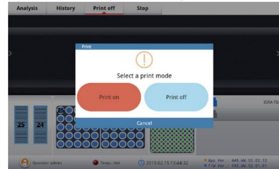
4. Make a choice to activate the print mode. If the print mode is on, the results of 3 tubes per a specimen are printed out when 3rd (Mitogen tube) test is finished.
