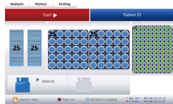
2. Adjust the number of test cartridges, tubes and tips on the touch screen. And make sure the activation of IGRA-TB ID chip.
